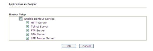
5. Open the DNSSD page again. The available items will be changed as the follows. It means the Vigor router (based on Bonjour protocol) is ready to be used as a printer server, FTP server, SSH Server, Telnet Server, and HTTP Server.
